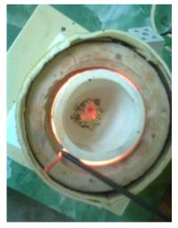
(e) Home-made furnace and temperature sensor(f) Annealing the gel at 500°CFigure 2 The synthesis processes of TiO<sub>2</sub>nanopowder
