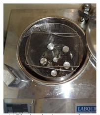
(c)Placing in the autoclave
