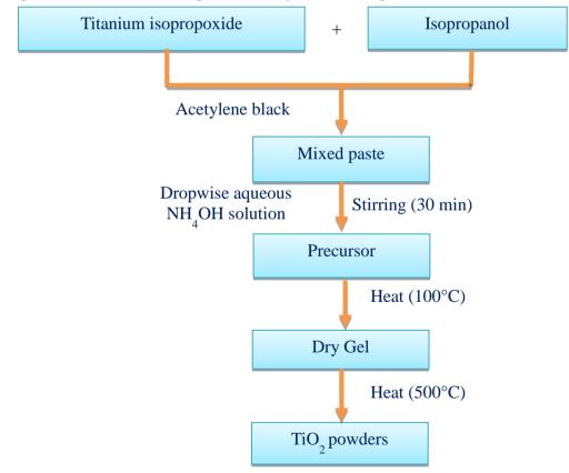
Figure 1 Flow scheme of the combustion process for the synthesis of NanocrystallineTiO<sub>2</sub> powders
