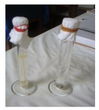
(a) Titanium isopropoxide and isopropanol
