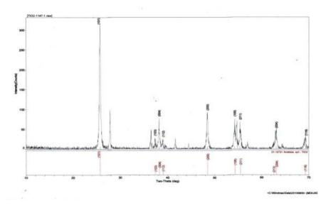
Figure 4 XRD pattern of TiO<sub>2</sub> nanopowders calcined at 500 °C
